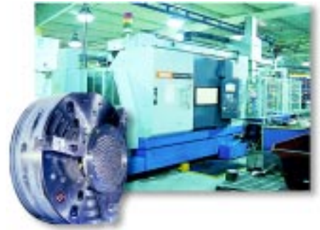
Robotic CNC Machining Center assures precision drilled tubesheets, twenty-four hours a day.
