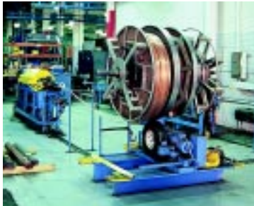
Use of rolled coil tubing supports the flexibility inherent in DFT manufacturing. Special straightening equipment and unique burr-free cutting process for superior rolled joints.
