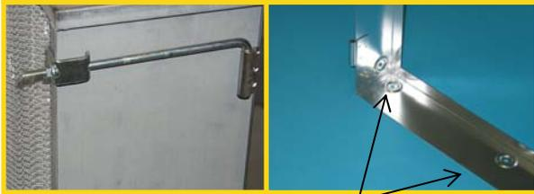
Swing bolts and equi-bearing clamps ensure an airtight filter to frame flange seal.
