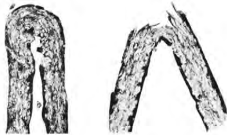
Figure 10-1. Effects of moisture content in folding paper. Sheet on left has proper moisture. Sheet on right lacks enough moisture—is dry and brittle—breaks on fold.
