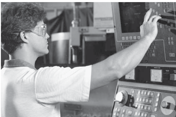
Computer-controlled equipment like this simplifies the process of drilling coil headers.
