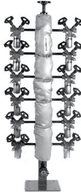
CCAF 212 Condensate Collection Assembly (Shown with TVS 4000 Trap Valve Station with 2000 Series Inverted Bucket all stainless steel steam traps with optional removable insulation package including nipples, drain valve and stand.)
