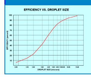
The Camfil Farr ECO® Moisture Separator is highly effective in removing water droplets, water mist and fog from outside or recirculated air. With an efficiency approaching 90% on 5-micron size droplets (98% on 20 micron size droplets) the ECO offers excellent protection of HVAC components including downstream filter banks. In addition, the ECO may be used downstream of DX or chilled water coils, and steam or mist-type humidifiers to allow saturated air to condense out of the airstream.
